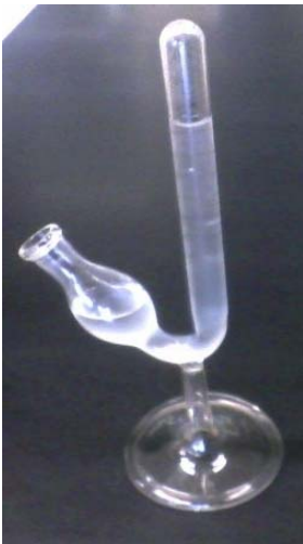
fig. 4-1 scilla peruviana yeast showing fermentation capacity in a Kühne's fermentation tube test
