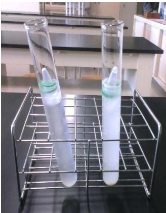
fig. 4-2 scilla peruviana yeast showing fermentation capacity in a Durham tube test (left : scilla peruviana, right : dry yeast)
