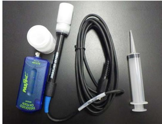
【Figure7】 Device to measure the amount of dissolved oxygen
